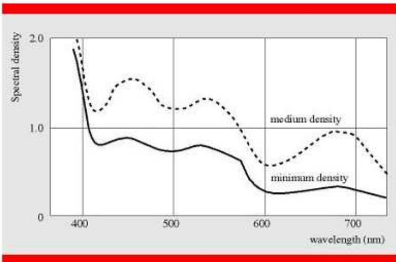
The curves show the spectral density measured on the processed image (neutral object with medium brightness), per wavelength. Standard processing.
