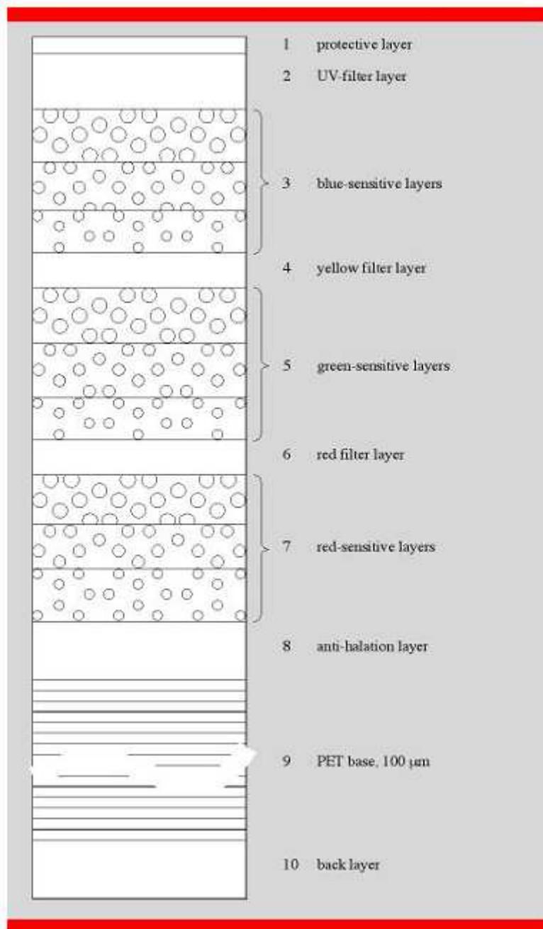
Total film thickness: 100 µm PET + 22 µm colour layers + 2 µm back layer = 124 µm.
