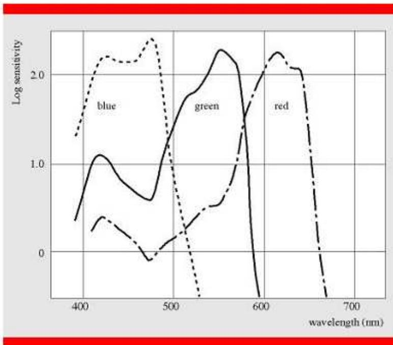
The curves refer to a density of 0.5 above base fog. The film is exposed to an equi-energetic spectrum. Sensitivity is reciprocal to the exposure expressed in  $\text{mJ}/\text{m}^2$ , required to produce the indicated density.
